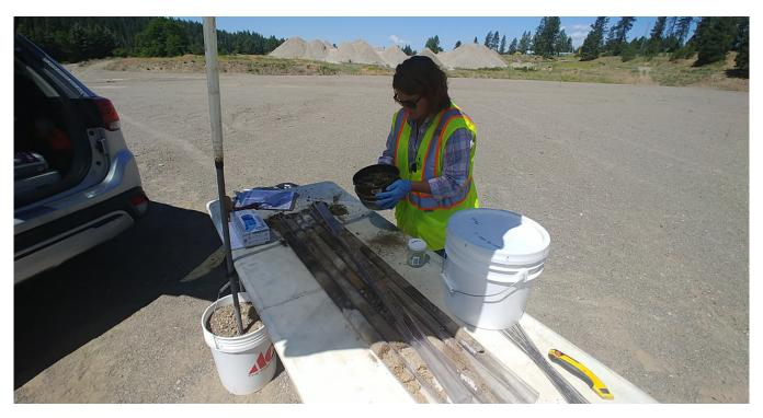
**Photo 3:** Looking west across DU-West during incremental sampling. DU-West occupies the western third of the Site. Shown are collected push-probe soil cores in Macrocore (PVC) liners and soil sieving.
