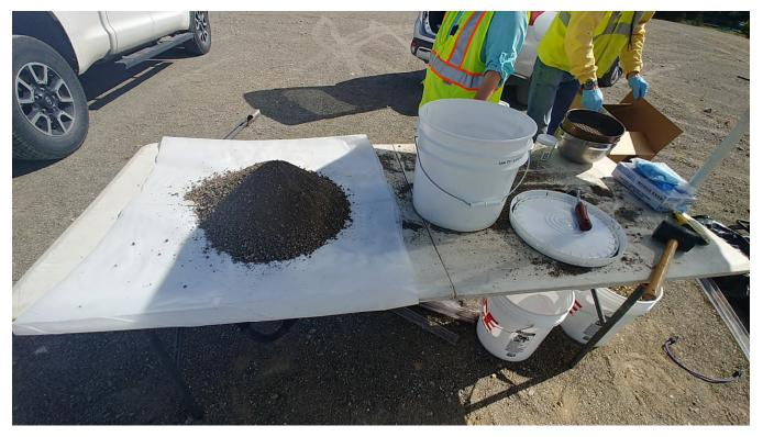
**Photo 4:** Looking at soil collected from DU-West. A cone of soil was created (cone-and-quarter process) in the effort collect a representative sample of homogenized and sieved soil for eventual PAH analysis.
